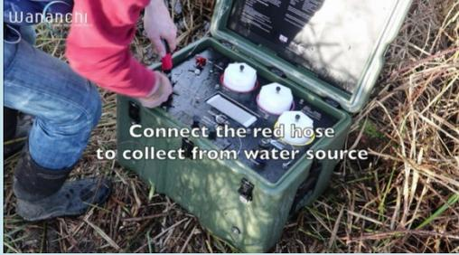
Connect the red hose to collect from water source
